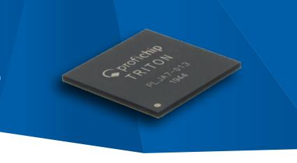
Triton combines industrial gigabit Ethernet communication with a fast and reliable backplane system as well as a powerful motion/automation multicore processor in one product with low power dissipation.
